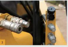
Free additional plugs for electronic attachments. The large-flow quick couplings will highlight their advantages in performance when using large-flow attachments.
